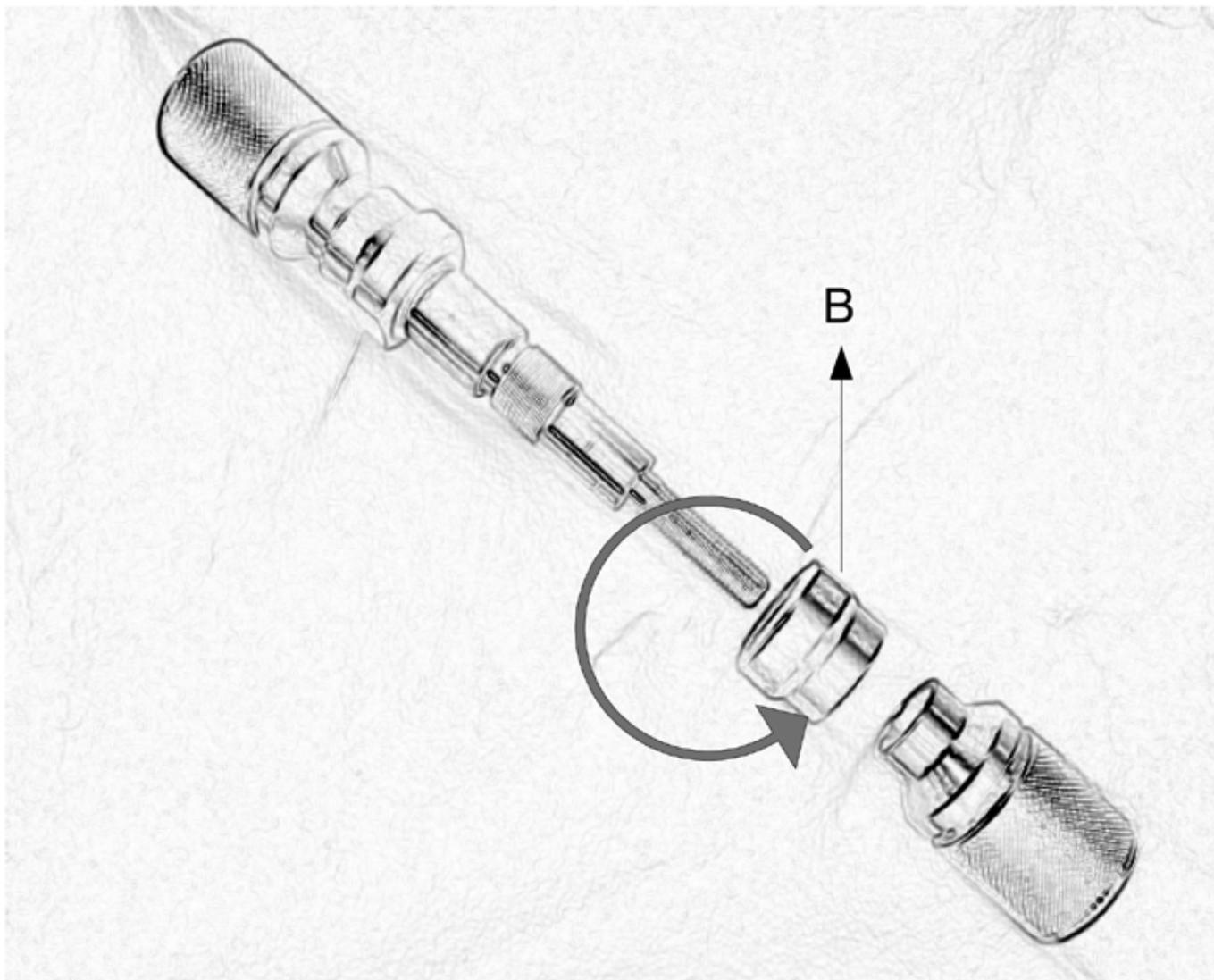
**4) EFFETTUARE LA STESSA OPERAZIONE SVOLTA PRIMA CON IL CORPO "A" ANCHE PER IL CORPO "B"**
